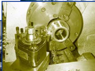
Turning 62HRC carbon steel with ceramics
